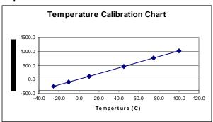
As you can see from the above table, with this board you will get an output of about 10.06 mV per degrees C. The values in the Est. column are values that were calculated from the linear regression equation that was derived from the Temp and MV data. Using that equation, the largest deviation (error) is 0.8 degrees C.
