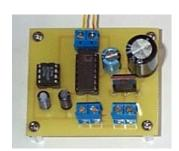
This circuit is based on the Analog Devices AD595 Thermocouple Amplifier. The nice thing about this chip is that it has on-board ice-point reference so there is no need to compensate for it. The output for these boards is 10mV per degree C. For instance, if you are measuring 15 degrees C, the output from this circuit will be 150 mV. –15 degrees C = -150 mV. If you use a DAC board with this, it must be able to handle these voltages.
